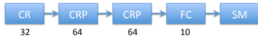
Figure 1. Basic neural network architecture used. CR is CONV-RELU, CRP is CONV-RELU-POOL, FC is fully connected and SM is a softmax classifier.
