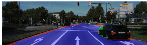
Figure 1. Training Image 01. Blue area is the correct prediction, red area is the false negative, and green area is the false positive.
