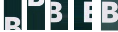
Figure 2. The first four images are augmented negative examples and the fifth image is the original positive example, with a centered B.
