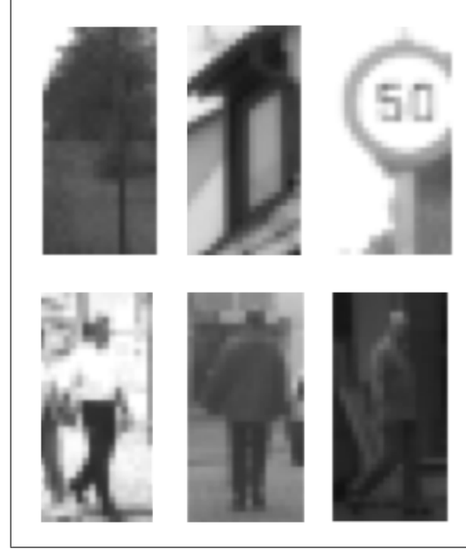
Figure 5. Negative and positive examples fed into the CNN classifier. Negative examples in the top row were extracted from the full-sized examples. Positive examples in the bottom row came directly from Daimler.
