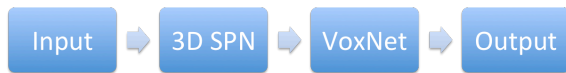
Figure 3: Architecture of 3D-SPN-VoxNet. The input is the 3D voxel data, and first go through 3D-SPN, then feed into VoxNet and get the output.
