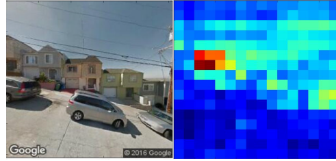
Figure 12: Inclusion heatmap showing the effect of only showing the network a region of the image on the class score
