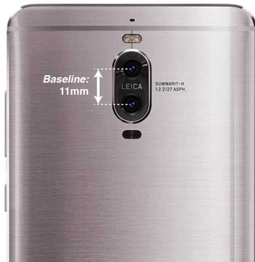
Figure 1. The device on which we conduct our final tests. It has RGB and monochrome sensors mounted with an 11 mm stereo baseline, and an ARM Mali GPU.
