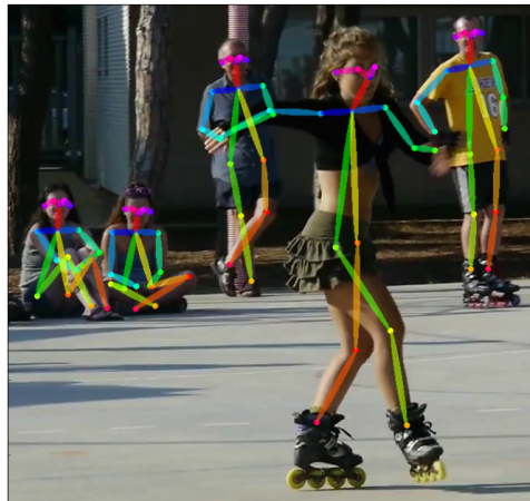
Figure 1. Example of output from Cao et al. 's convolutional network. Their work focused on improving multi-person pose estimation, but still performs very well on images of individual persons.
