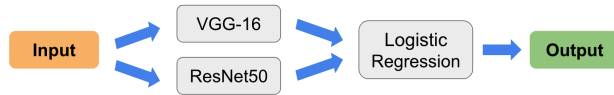
Figure 3: Ensemble learning architecture with VGG-16 and ResNet50 as input models into the logistic regression ensemble model for final predictions.
