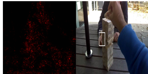
Figure 12. Saliency map of a mislabeled image where lots of background pixels are picked up.
