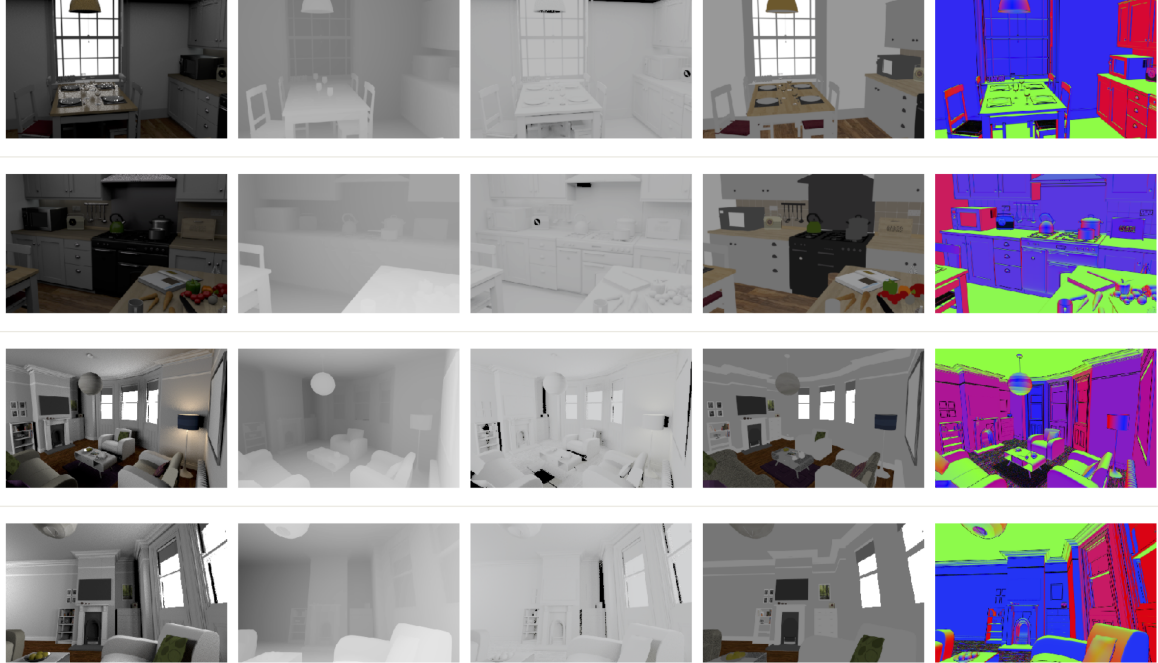
Figure 1. From left to right: original image, depth map, log-normalized light intensity map, approximated diffuse material map, and normal map.
