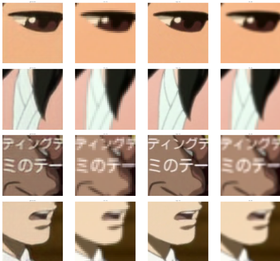
Figure 8. 4x GAN example validation results after training. From left to right: Generator outputs, low-resolution generator inputs, high-resolution ground truth images, bicubic upscale
