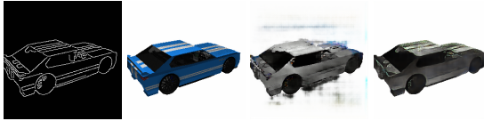
Figure 8: Validation output trained with transpose convolution and resize convolution. Resize convolution greatly reduces the checkerboard artifacts. From left to right: edge input, ground truth, output with transpose convolution, output with resize convolution.
