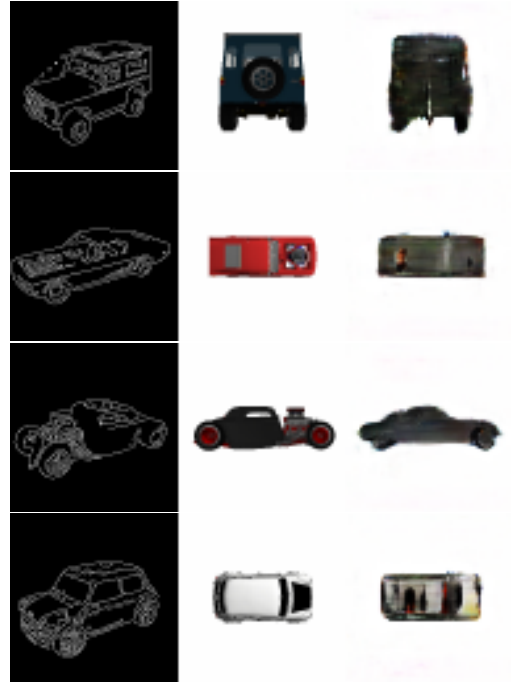
Figure 19: Failure cases of Multi-View Architecture I model. From left to right: edge input, ground truth, our output. Common failure cases include: asymmetric "back" view outputs, missing details and patch artifacts causing outputs that don't look smooth.
