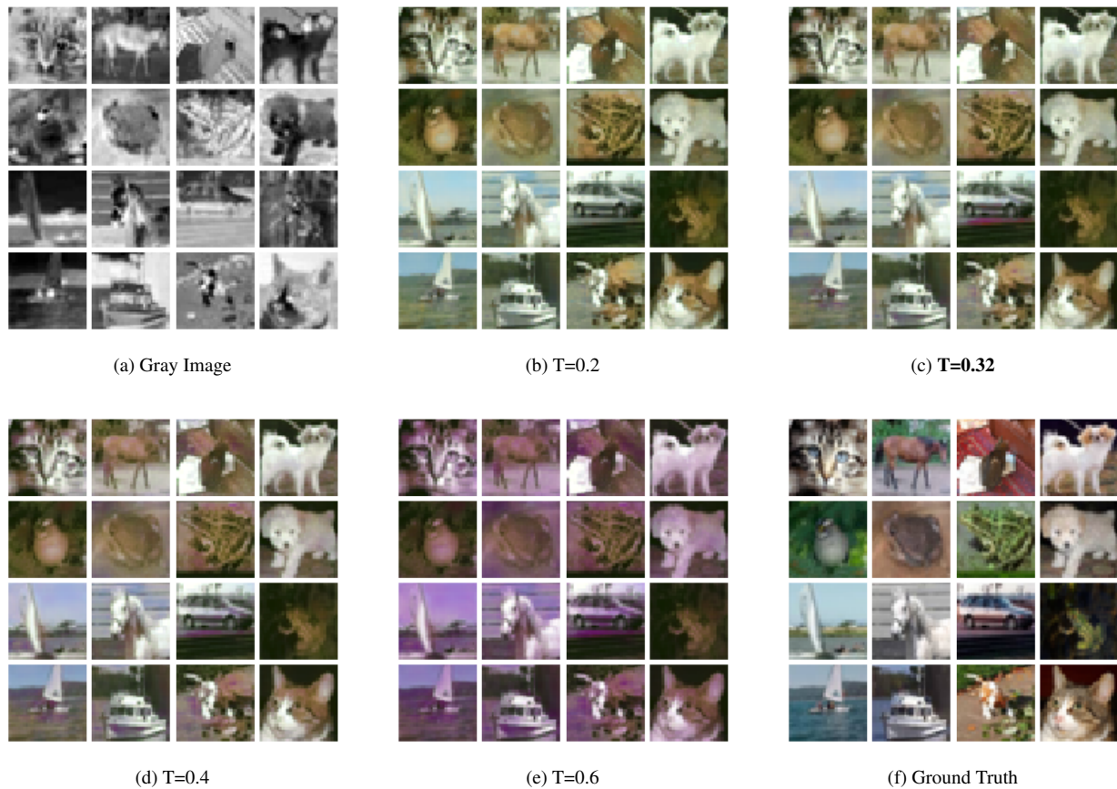
Figure 6: Random sample of 16 images from their test set. Figure 6a shows the grayscale version, the next three figures show colorization produced by classification model for different values of T, figure 6f shows ground-truth
