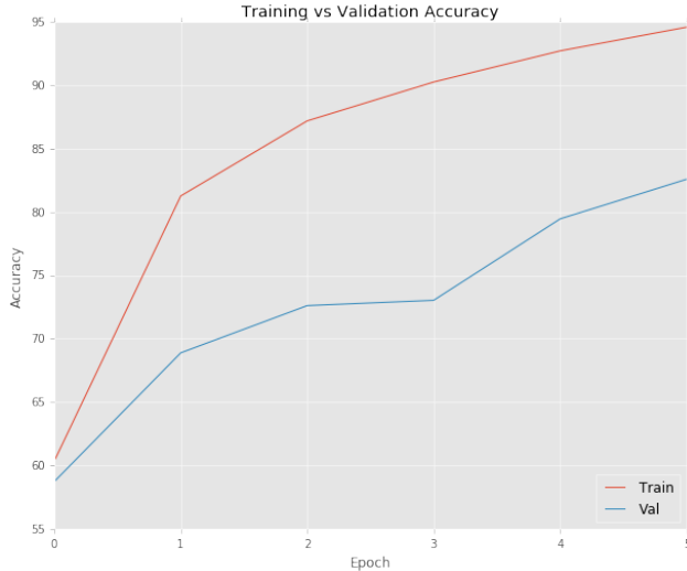
Figure 11: A comparison of the classification accuracy in the training and validation sets for our 3D-CNN model across a single viewpoint (frontally facing the bed) on ternary classification.
