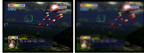
Figure 3. An original 480 \times 640 frame (left) compared to a compressed 48 \times 64 frame (right).
