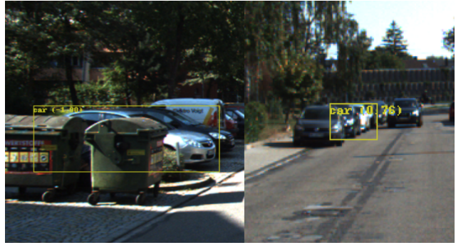
Figure 11. Failure Mode: Partially Blocked Object
