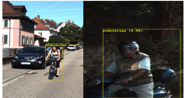
Figure 12. Failure Mode: Confusion Between Pedestrians and Cyclists
