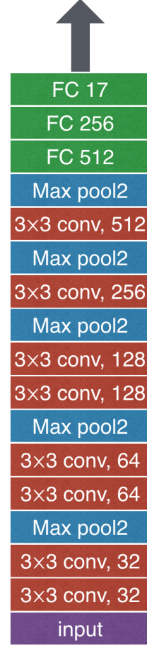
Figure 5. Convolutional neural network architecture. Eleven convolutional or fully connected layers are used in total. We use ReLu activation function, batch normalization and dropout for each convolutional or fully connected layers.
