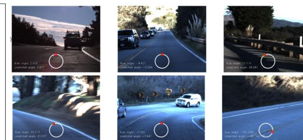
Fig. 6. Prediction visualization of steering angles. The green circle indicates the true angle and the red circle indicates the predicted one.
