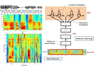
Raw speech features (left column) are computed by Fourier Transform of each short frame (25 ms), and grouping to 40 perceptual frequency channels by a filterbank. A speech waveform is converted to a time-frequency (TF) plane.
