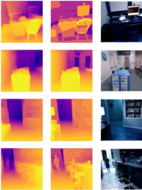
Figure 7. Depth maps results of transfer learning based model. Starting from the left column is the predicted depth map, one in center is true depth and on the right is an original image.
