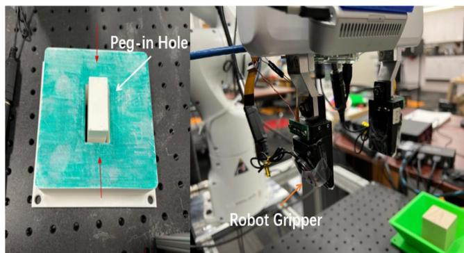
The visual encoder built in this project should guide a given controller to learn and perform peg insertion shown above. The data set includes a series of images of the robot's workspace and corresponding ground truth actions (human demonstration). Since the action space of the robot is discrete, the evaluation metrics are cross entropy loss and accuracy.
