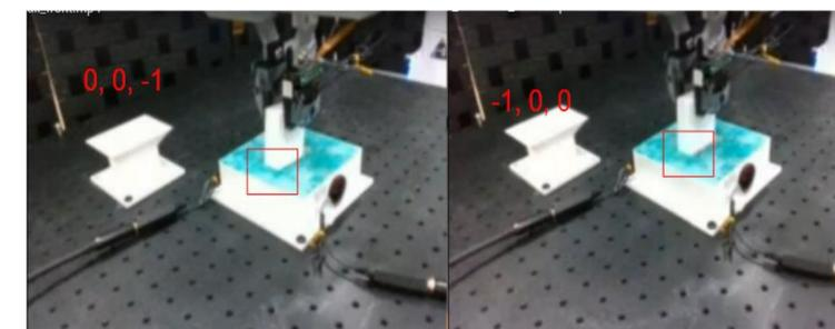
We performed 50 real-robot test with each trail starting at a random initial position. If the peg is inserted in the hole in the end, we will count it as a successful case. Finally, our model achieves a success rate of 84%. In the failure cases, the model predicts the wrong action at the edge of the hole base. This is because there is some vague representation in the vision
