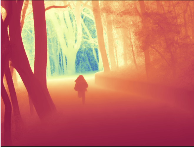
Figure 5: Generated Depth Map by the Modified Marigold Model where darker colors indicate objects perceived by the model to be closer
