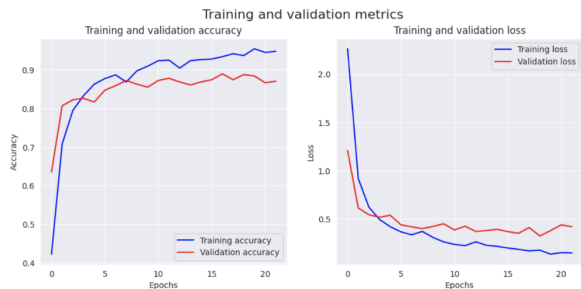
Figure 11. Validation and training curves for accuracy (left) and loss(right) of the ResNet152-V2 model
