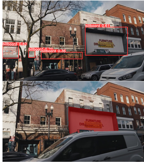
Figure 3. YoloV8+SAM for billboard detection and precise mask segmentation.
