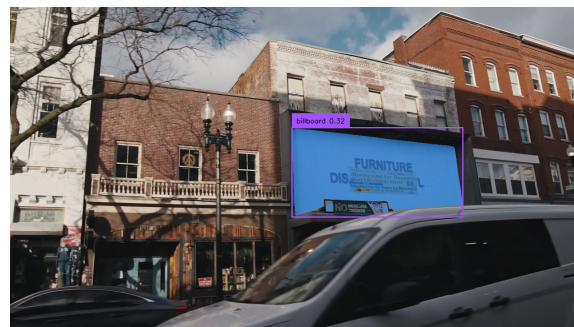
Figure 4. GroundedSAM for billboard detection and precise mask segmentation
