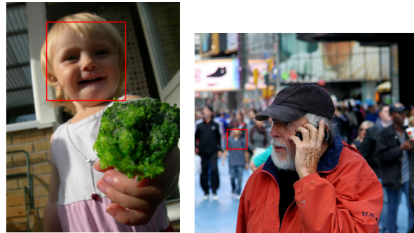
Figure 4. Face detection examples using Haar Cascades and a common failure faced. On the left, a face is correctly detected, while on the right, there is a false positive and a false negative. In the false positive, an incorrect bounding box is constructed in the background, and in the false negative, the main face is not correctly detected.
