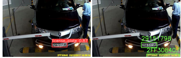
Figure 3. Output from YOLO-V8 (left) and EasyOCR (right) on the same image for license plate detection. Note that EasyOCR also flags the timestamp of the image.
