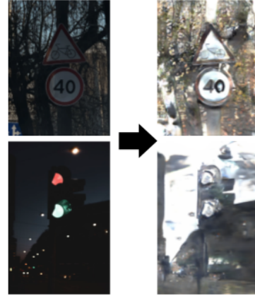
Figure 3: Examples of Converting Night Images (Left) to Fake Day Images (Right)
