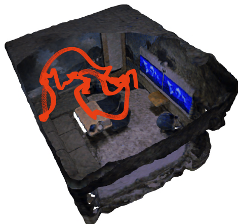
Figure 2. Estimated environment mesh and camera poses produced by 3D SLAM
