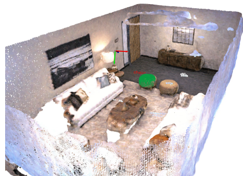
Figure 7. Chair segmentation mask (green) projected into 3D world coordinates, with object label above it (red)
