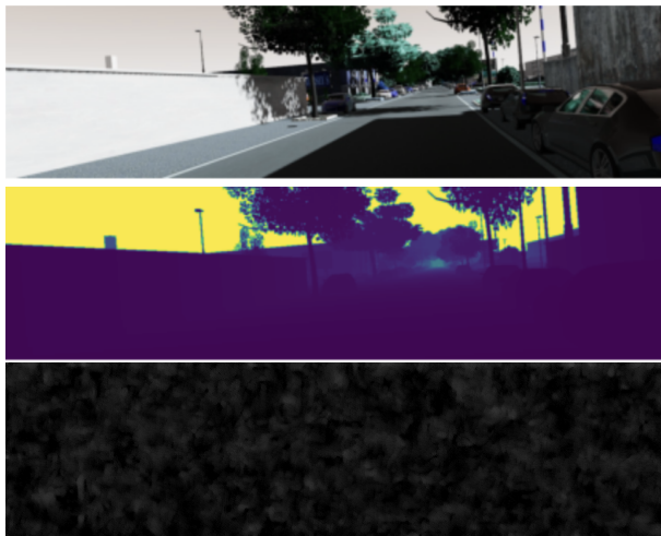
Figure 5. Top: An RGB image from Virtual Kitti 2. Middle: The corresponding ground truth depth map. Bottom: The generated depth map from our LDM.
