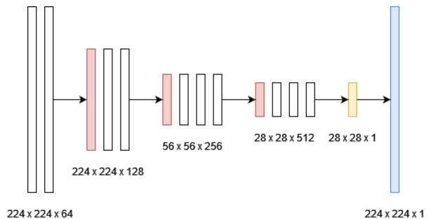
Figure 1. Diagram of an FCN block. Red represents 2 \times 2 max-pooling layers. Yellow represents a 1 \times 1 convolution layer. Blue represents an upsampling layer. All other unmarked layers are convolutional layers with a kernel size of 3 and padding of 1, followed by batch normalization and ReLU activation. Text labels denote the output size of the convolutional layers.
