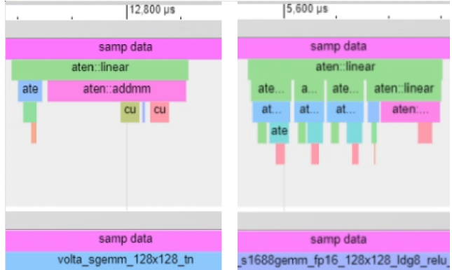
Figure 4: 4096 \times 4096 Linear Layer in MLP. This shows the execution traces (Left: FP32, Right: FP16) for a forward pass through one linear layer of input size of 4096 and output size of 4096. With larger linear layer size, we now see the GPU spending more time doing the computation according to the bottom bar, hence increasing the GPU utilization. Higher GPU utilization allows for the hardware speedup benefit to become more visible.
