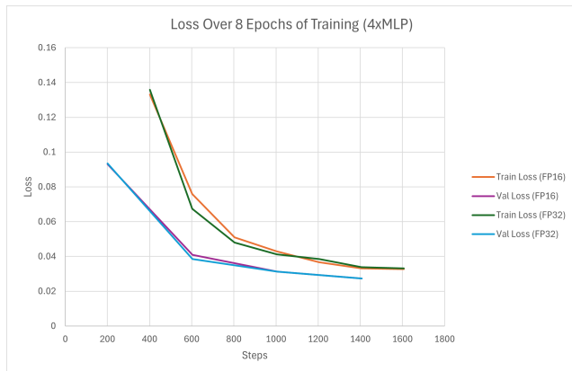
Figure 5: Training loss and validation loss for training the modified 4xMLP HuMoR model using FP16 and FP32 over 8 epochs.
