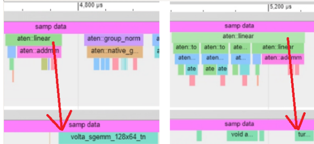
Figure 3: 1024 \times 1024 Linear Layer in MLP. This shows the execution traces (Left: FP32, Right: FP16) for a forward pass through one linear layer of input size of 1024 and output size of 1024. The red arrow indicates the corresponding GPU kernel for the linear layer, where the computation are being done. Everything before is overhead logic to copy the data into GPU and, for FP16, also logic to convert FP32 data to FP16.
