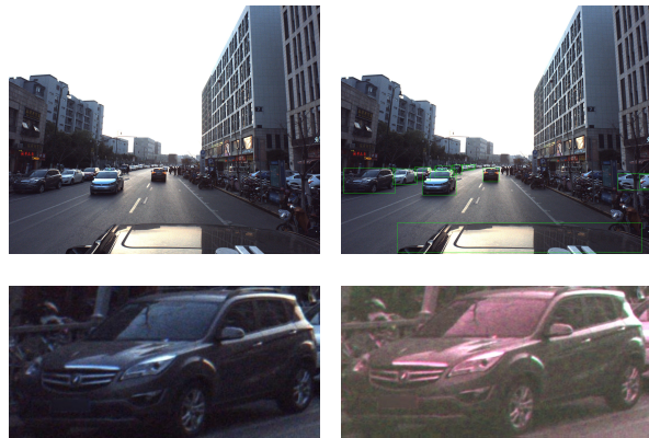
Figure 3. Data Processing Example. Top Left: Original Image. Top Right: YOLO Output. Bottom Left: Cropped Image based on bounding boxes. Bottom Right: Augmented Image.
