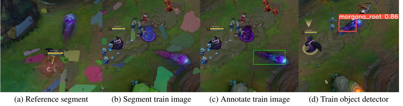
Figure 2. Dataset creation and finetuning object detection. (a) First, we segment each frame and choose a single (or small number of) frame(s) where the projectile is visible. We use the corresponding object mask to compute heuristics \mathcal{H} . (b) Now, to prepare the dataset, we segment each of the train/val/test images and (c) computationally identify and annotate the objects of interest using similarity in the heuristics \mathcal{H} . (d) We now finetune the YOLO object detector to detect projectiles, informing the player of the correct movement input to dodge.
