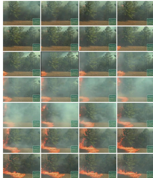
Fig. 6 - Sequence of frames extracted from a video of a developing fire, with a 2-second interval between each frame. Our model successfully detected the presence of fire in the 10th frame, highlighted with a black border, illustrating the model's capability to recognize fire as it becomes a more prominent feature within the frame.
