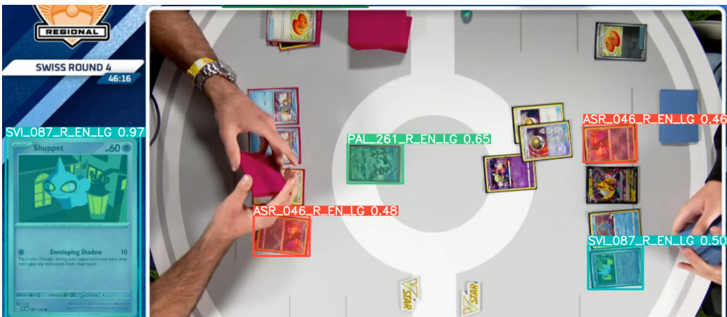
Figure 12: Detection using Preprocessing + Mosaic + Mask Clipping model.
