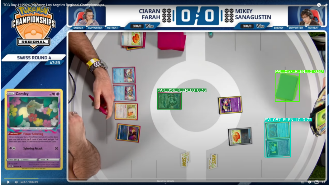
Figure 10: Detection using Preprocessing model. Notice how a card sleeve is erroneously detected a Pokémon, and two cards are detected as one.
