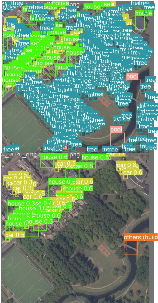
Figure 1: This example of labels (top image) compared to predictions (bottom image) shows that the YOLO model can correctly predict some classes, but struggles with some dense objects like trees.
