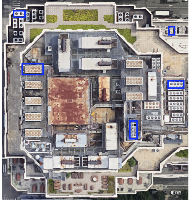
Figure 1. Overhead aerial imagery of a commercial building in New York City, with some examples of RTUs outlined in blue. Other rooftop features such as greenery, ducting, seating, and tiling also clutter the scene.
