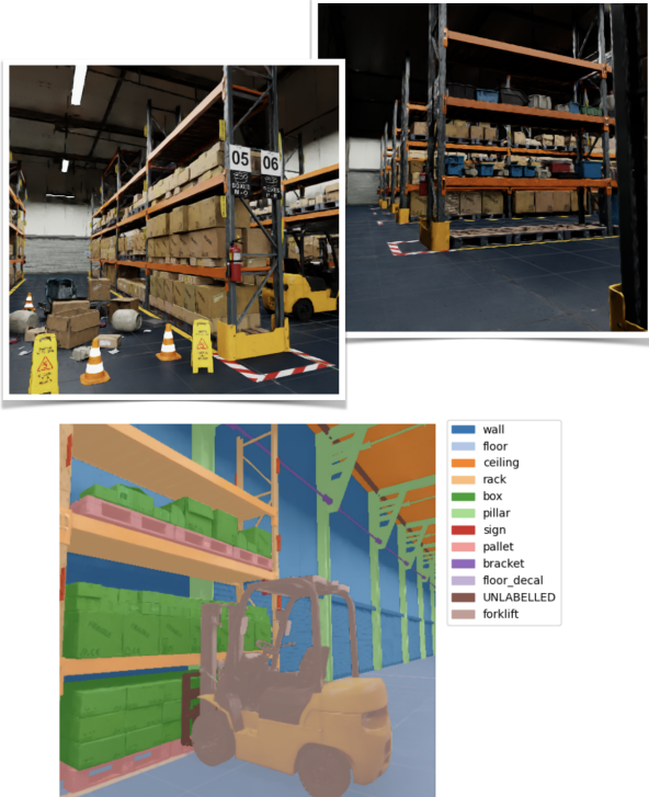
Figure 3. Samples from the generated synthetic dataset. Top: RGB images, showcasing the photo-realistic fidelity of ISAAC Sim. Bottom: overlay with ground-truth segmentation data generated via the Synthetic Data Recorder tool.
