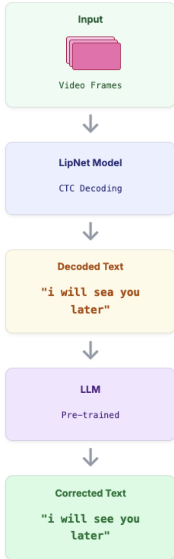
Figure 3. High level block diagram of how a fine tune LLM can be used after a Visual recognition block model output for better prediction accuracy
