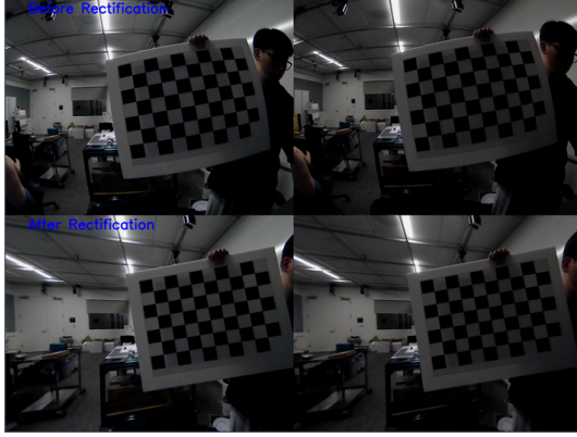
Figure 1: (Top) Raw fisheye camera input with barrel distortion. (Bottom) Undistorted and rectified image used for stereo depth estimation.
