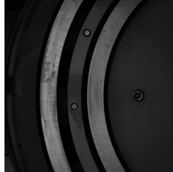
Figure 1: example bruised bearing surface
