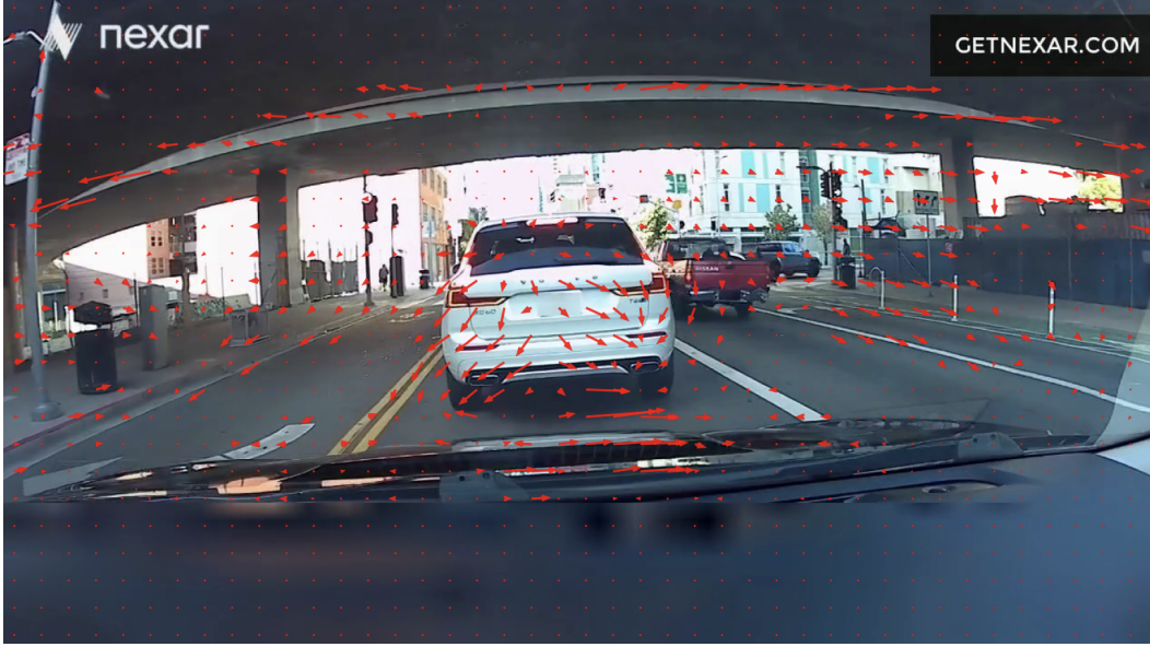
Figure 2. A visualization of the optical flow fields obtained from a pair of frames from a video in the training set. The arrow length is proportional to a pixel’s estimated movement between frames.
