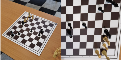
Figure 4: Homographic transformation used to flatten the board to a top-down view.
