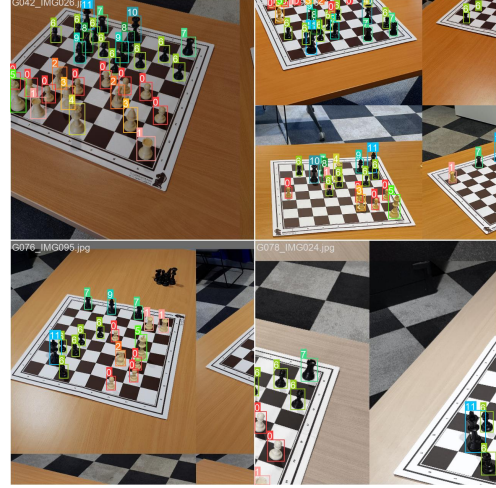
Figure 8: Example of a training batch with mosaic augmentation and horizontal flipping.
