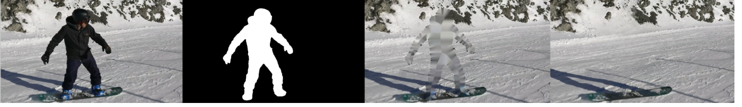
Figure 2. On the far left we have the input image, second we have the segmentation mask generated by SAM-H, third we have the background inpainting provided by OpenCV, and on the far right we have the inpainted background generated by LaMa MultiPass.
