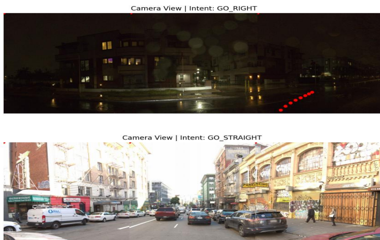
Figure 4: Failure cases: Top: Under low-light and rainy conditions, the model fails to predict a correct right turn, likely due to degraded visibility from glare, reflections, and water droplets on the lens. Bottom: In a dense urban environment, the model fails to predict the correct trajectory, potentially misinterpreting nearby pedestrians, moving and parked vehicles
