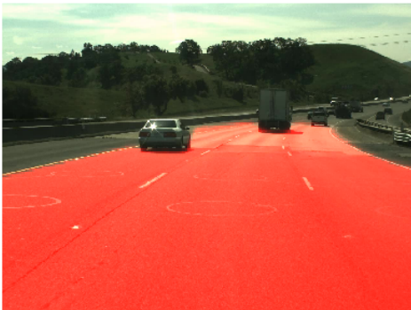
Figure 5. The red shaded regions show the softmax score of the correct class for that pixel patch in the image. The network successfully predicts the open road surface as free space. Notice that the road shoulder on both sides are not labelled as free even though these two areas are visually very similar.
