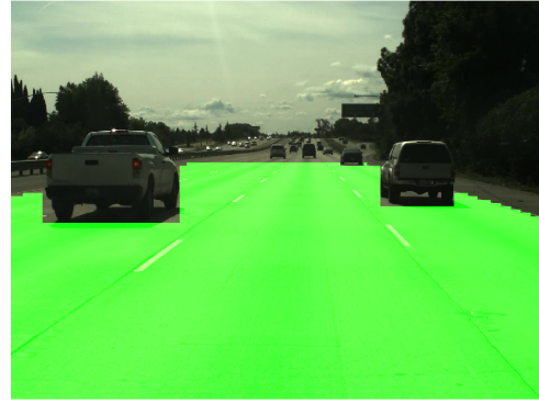
Figure 3. Example of combined car and lane labels showing free road surface label. The green shaded areas show the area of image labelled as free space.
