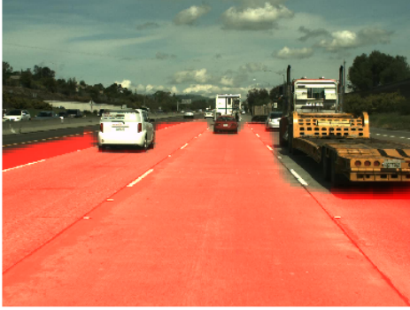
Figure 4. The red shaded regions show the softmax score of the correct class for that pixel patch in the image. The network successfully predicts the open road surface as free while indicating the truck and vehicles as not free space.
